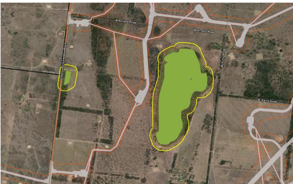
Figure 7.4 Outcome of design to show complete avoidance of HES wetland areas (green), including a 100 m avoidance buffer (yellow)
