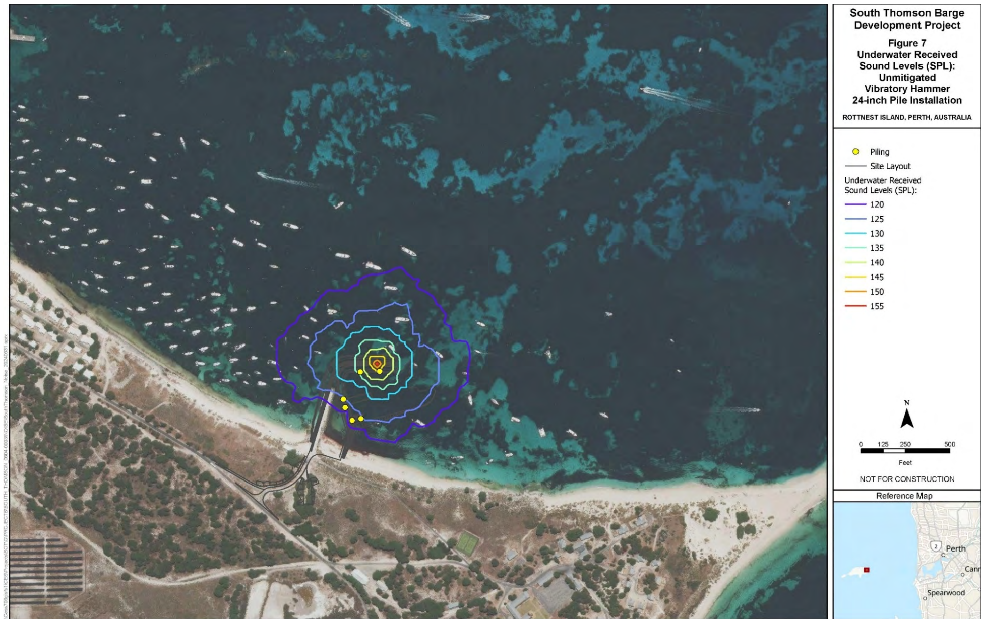
Figure 36: Underwater Received Sound Levels (SPL): Unmitigated vibratory 24-inch pile installation (proposed piling method)
