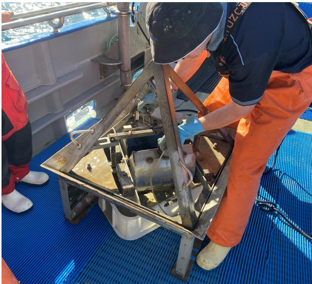
Figure 10. The Ponar grab operated from the winch on board the research vessel.
