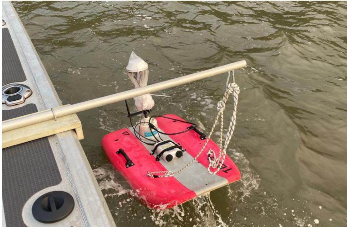
Figure 5-3 ADCP Setup attached to boat
