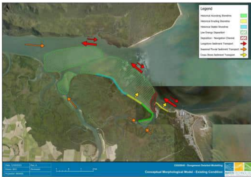
Figure 3.1 Conceptual model of existing sediment transport processes (Water Technology 2024a).
