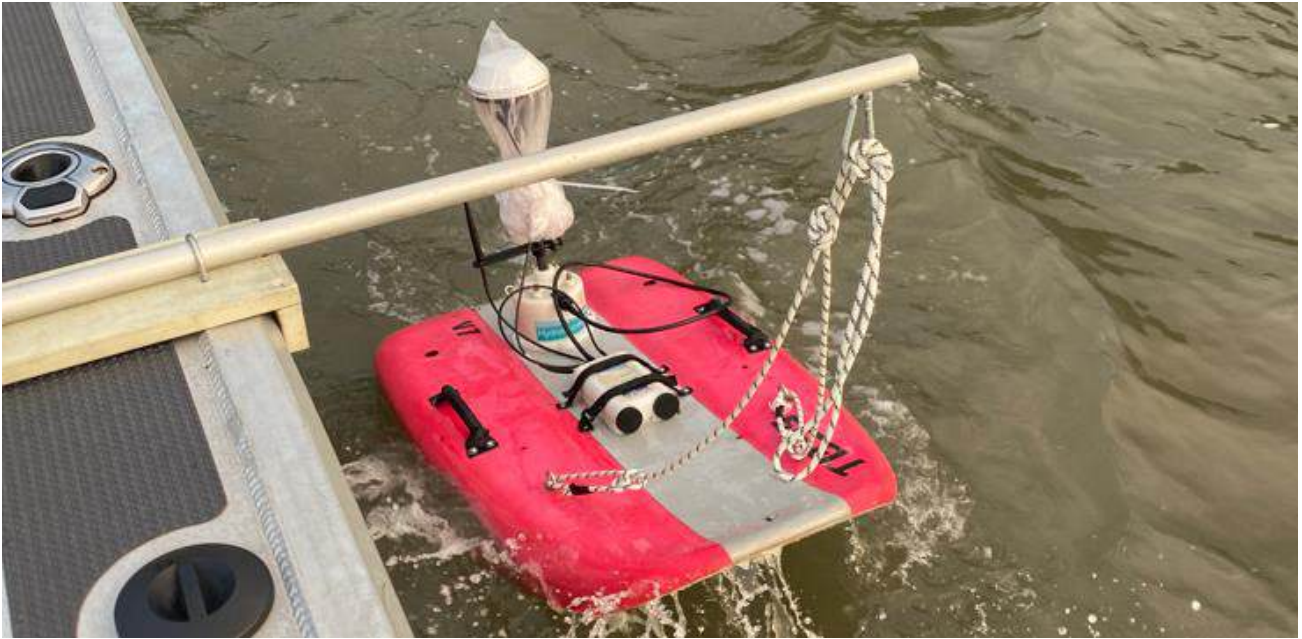
Figure 3-6 ADCP Setup attached to boat
