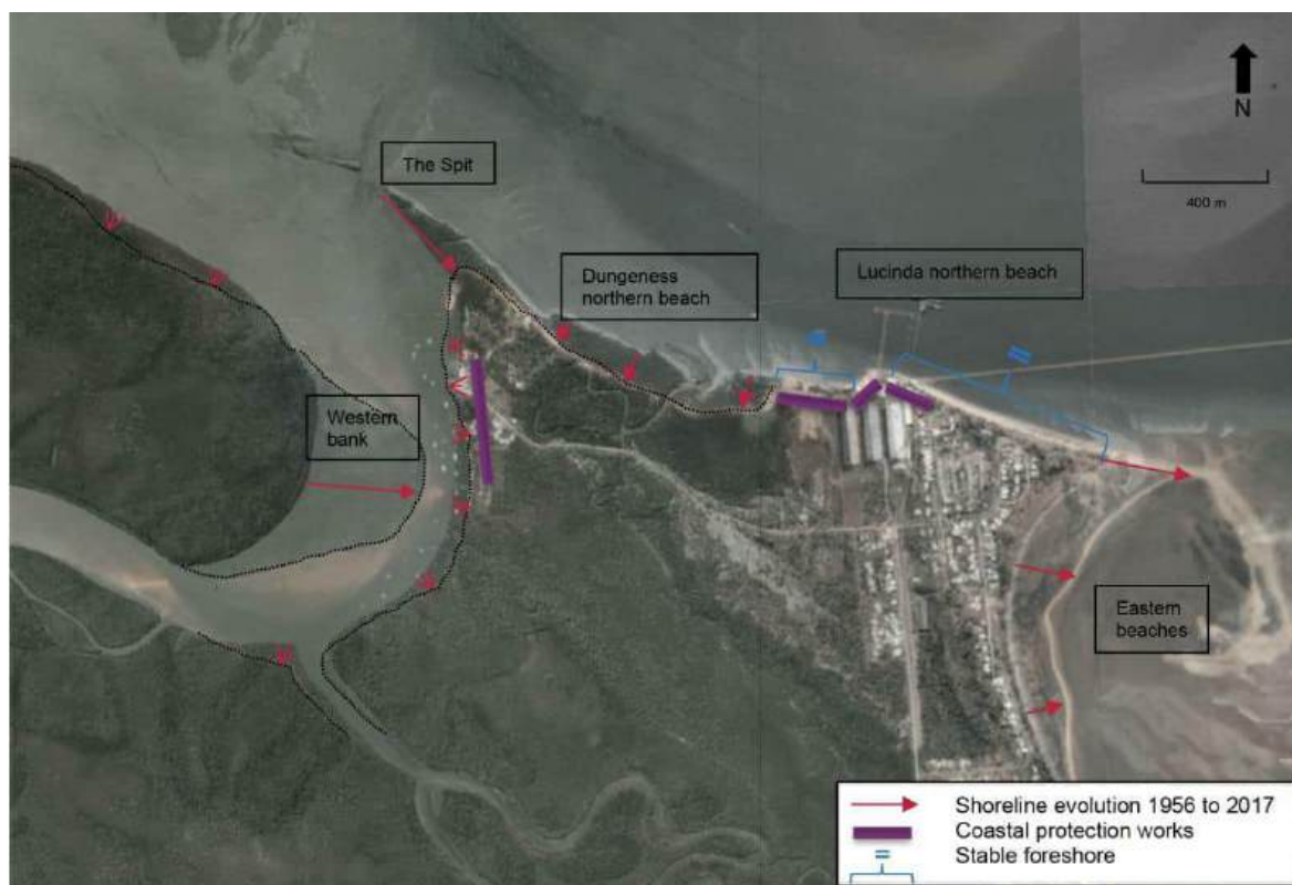
Figure 2.2 Aerial imagery from 1956 and 2017 (dotted outline) showing significant erosion of the spit and the northern foreshore of Dungeness (Water Technology 2019).
