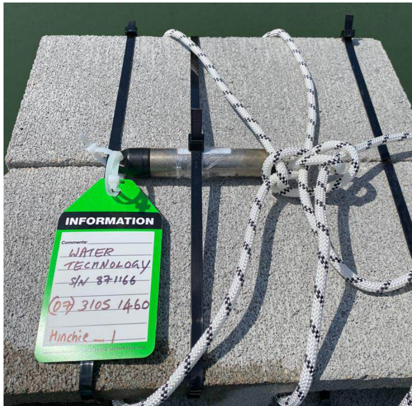
Figure 5-2 Water level logger and deployment mount
