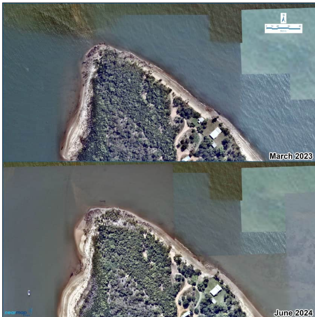
Figure 12: Shoreline erosion and mangrove loss along the foreshore
