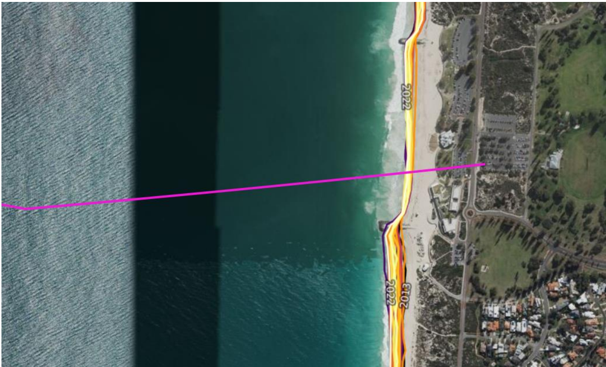
Figure 2.4 Annual shorelines and rates of coastal change from 1988 – 2021 in the vicinity of City Beach. Source: DEACoastlines, Geoscience Australia, accessed October 2023 (1:25,000 base map)
