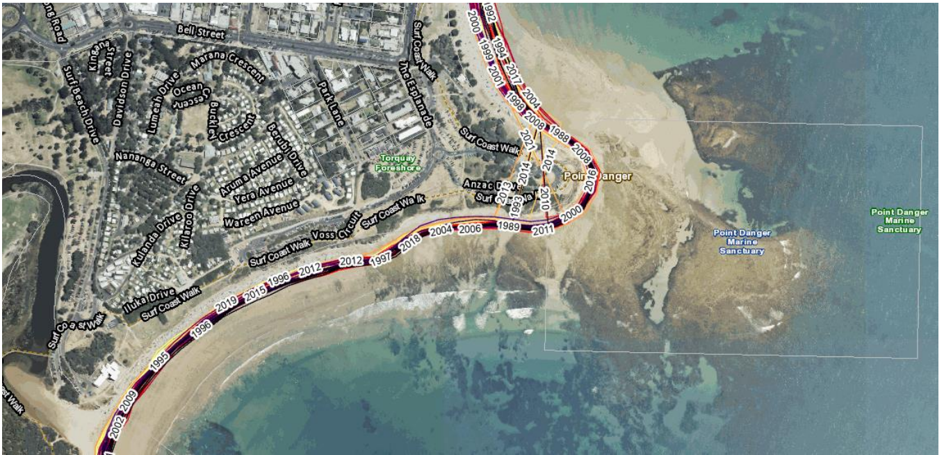
Figure 2.27 Annual shorelines and rates of coastal change from 1988 – 2021 near the Voss' Circuit site. Source: DEACoastlines, Geoscience Australia, accessed December 2023 (1:2500 base map)
