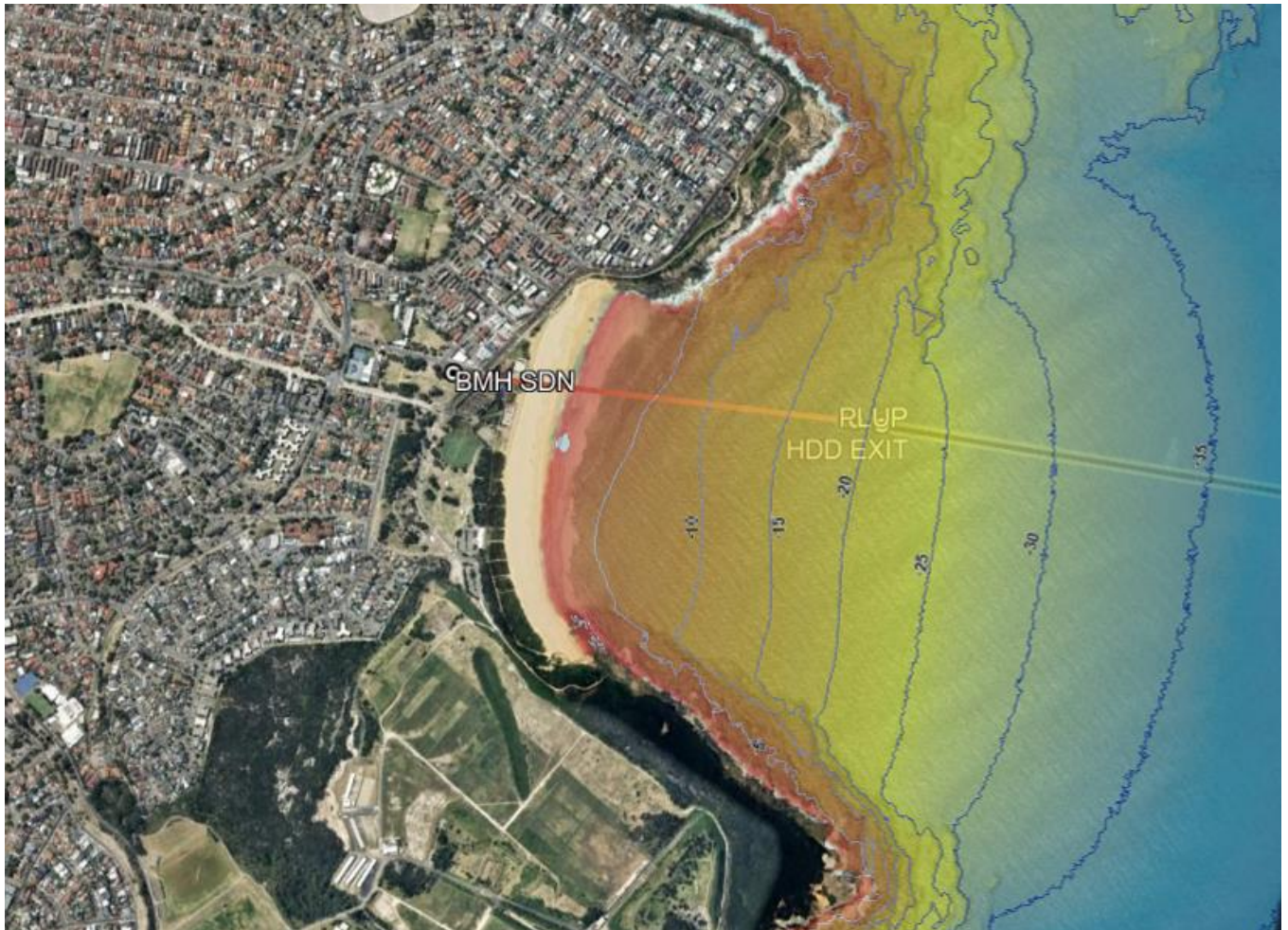
Figure 2.28 Bathymetry at Sydney Maroubra landing to -35m contour. Pink line depicts proposed route (GHD Esri maps overlaid with NSW Marine Lidar Bathymetry Data 2018 DEM [SEED, https://www.seed.nsw.gov.au ])
