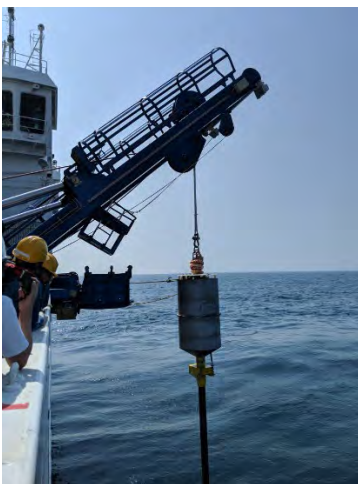
Figure 3.6 Example of piston coring equipment (left, courtesy of OSIL) and cone penetrometer test equipment (right, courtesy of EGS)
