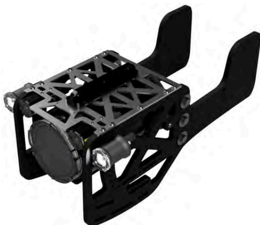
Figure 3.8 Example of a DDV camera used for benthic habitat mapping (Source: Spotx, 2024)
